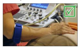
Consider a cable brace to eliminate the pull from the cable
